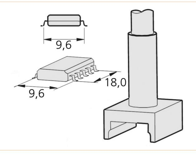
SMD Desoldering Tip Series C245 for Soldering Iron T245 (formerly AD-2245)
