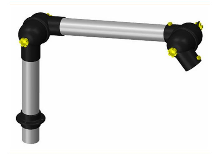
The Alsident 50 system has tubes with a diameter of 50 mm and is suitable for air volumes of 45 -85 m3/h. As a result, the system is ideally suited for use in industries with smaller detection tasks, such as the electronics industry, laboratories, laser technology or even for specialist rooms in schools. The ESD-compliant extraction arm naturally complies with DIN EN 61340-5-1 and is earthed with  $1M\Omega$  resistor.
