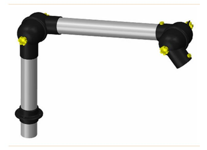
The Alsident 50 system has tubes with a diameter of 50 mm and is suitable for air volumes of 45 -85 m3/h. As a result, the system is ideally suited for use in industries with smaller detection tasks, such as the electronics industry, laboratories, laser technology or even for specialist rooms in schools. The ESD-compliant extraction arm naturally complies with DIN EN 61340-5-1 and is earthed with  $1M\Omega$  resistor.
