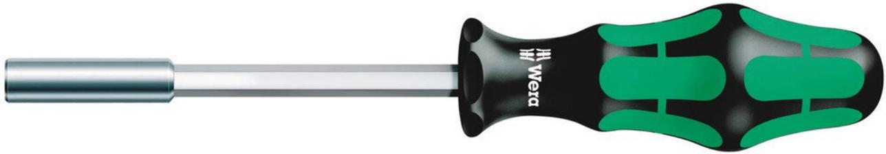
Bit holder with Kraftform Plus handle for comfortable ergonomic working, preventing blisters and calluses. Hard grip zones for high working speed, while soft grip zones guarantee high torque transmission. The integrated snap ring guarantees that the tool sits perfectly in the holder. Suitable for bits with 1/4" external hexagon drive to DIN ISO 1173-C 6.3 and Wera connection series 1.
