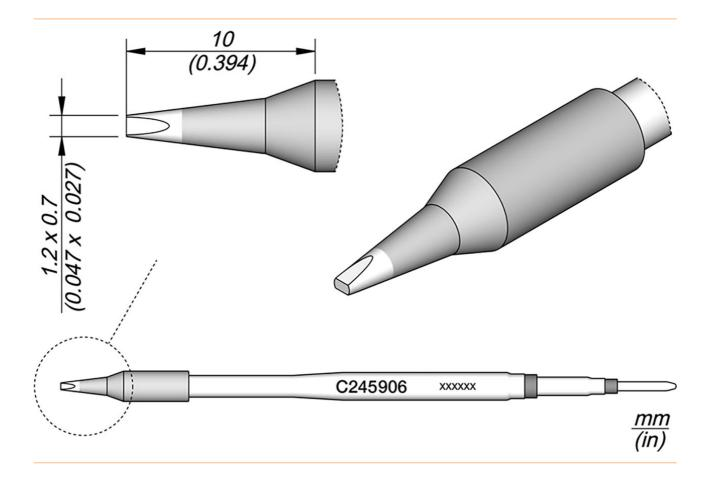
Soldering tips series C245 for soldering iron T245 (formerly AD-2245). They are suitable for general soldering purposes. Sleep and sleep mode in the clipboard.
