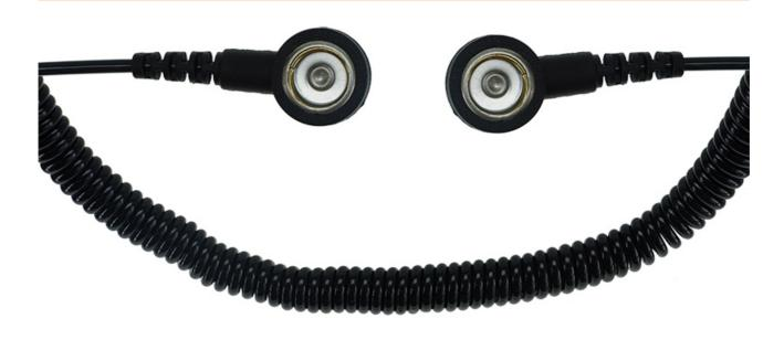
The ESD spiral cable from Safeguard is an important component in personal grounding in the ESD zone (EPA) to protect electronic equipment and components from electrostatic discharge. The leakage resistance is 2x 1 Mohm. The length of the cable of 2.4 meters allows flexible working without restricting the freedom of movement. The ESD spiral cable in black color has 2x 10mm push buttons. The color scheme allows the cable to be easily recognized at any time and in different lighting conditions.
