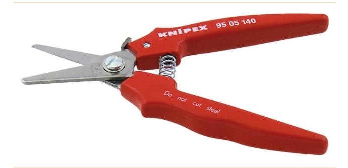
For cutting cardboard, plastic, Al, Ms and Cu foils. Not suitable for steel wire and sheet iron. Hardened cutting edges with precision grinding. With opening spring and ratchet. Clamp protection prevents crushing injuries. Adjustable screw joint.
