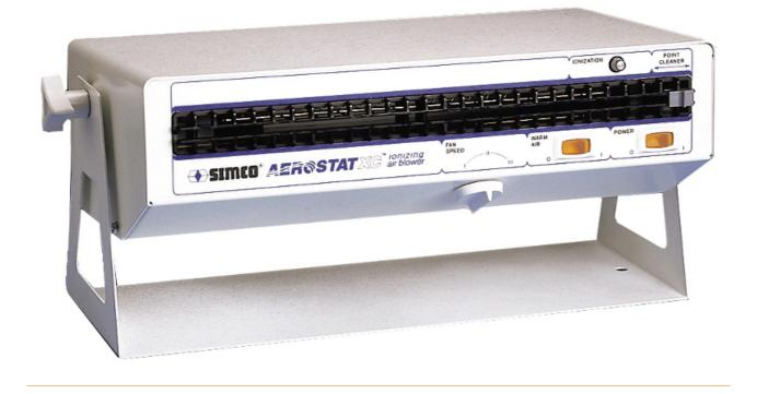
With the ESD ionizer Aerostat-XC from Simco, electrostatic charges can be neutralized at ESD workstations. The blower of the Aerostat-XC consists of three fans with infinitely variable speed control and switchable heating element, which can be heated up to an ambient temperature of 6°-8°C. The blower can be switched on and off at any time. Ionization is based on high voltage (AC alternating voltage technology). Very low maintenance requirements.
