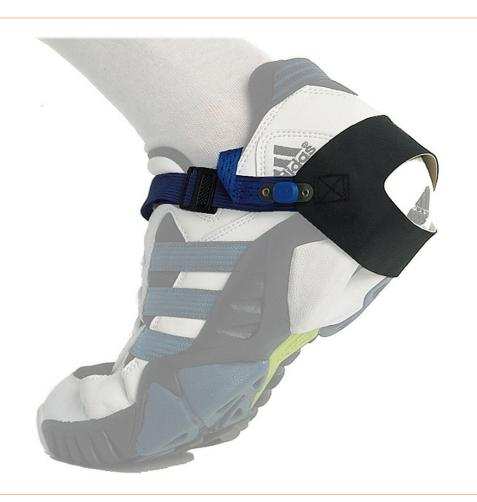
The ESD heel strap from Safeguard is an important accessory for correct personal grounding. It has a leakage resistance of 1 MOhm and a clip closure. The heel strap is designed to dissipate static electricity from the feet, preventing damage to electronic equipment and components. The 1 MOhm leakage resistance ensures that the dissipation of static electricity is effective and safe. The tape ihat the color black and adjusts to the size of the feet.
