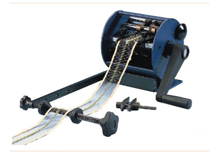
Bending and cutting device for axial components Finished stand-up axial components
