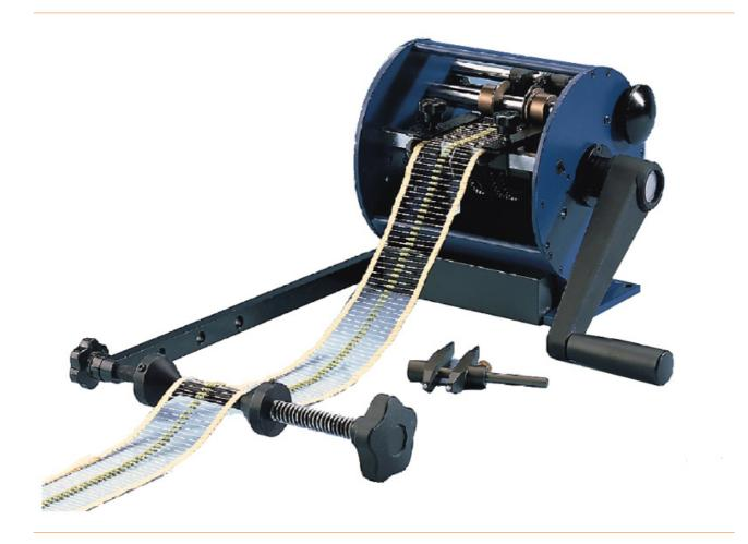
Bending and cutting device for axial components
