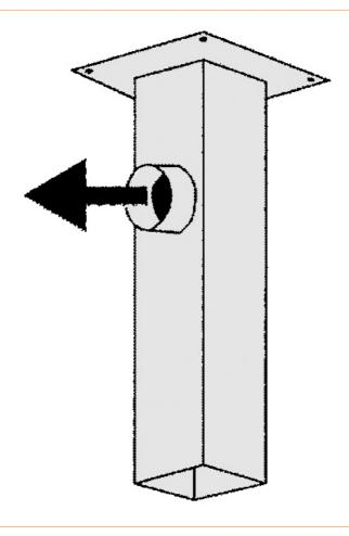
With the base boxes from Alsident the installation of the extraction arms for ceiling mounting is very easy to accomplish. These are made of steel and are painted with TGIC powder paint on all surfaces.
