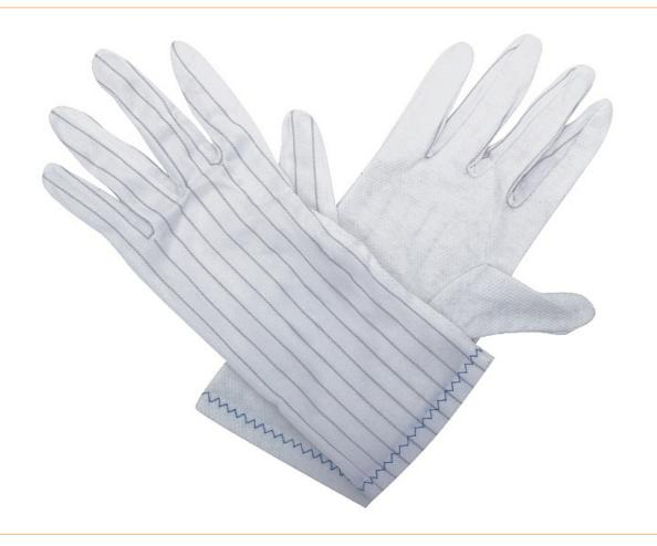
These ESD gloves from Warmbier offer your employees effective all-round protection against electrostatic discharge when working with sensitive electrical components in an EPA. The conductivity of the gloves is achieved by the conductive special fibre carbon, which is incorporated in the glove liners.
