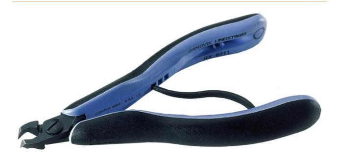
Made of high-performance ball bearing steel, burnished. Cutting and jaws computer-ground, thus highest precision and constant quality. Induction hardening of the cutting edges to 63-65 HRC. Handles of 2 components, with opening spring.
