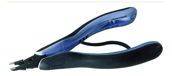
Made of high-performance ball bearing steel, burnished. Cutting and jaws computerground, thus highest precision and constant quality. Induction hardening of the cutting edges to 63-65 HRC. Handles of 2 components, with opening spring.
