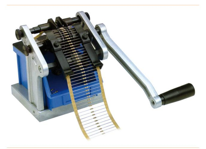
Cutting and bending device for axial components Cutting and bending on both sides
