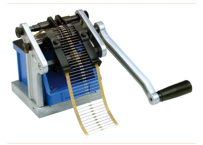
Cutting device for axial components
