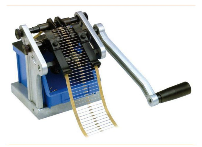
Cutting and bending device for axial components Cutting and bending on one side, cutting only on other side
