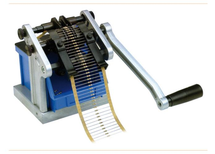
Cutting and bending device for axial components Cutting and bending on one side, cutting only on other side
