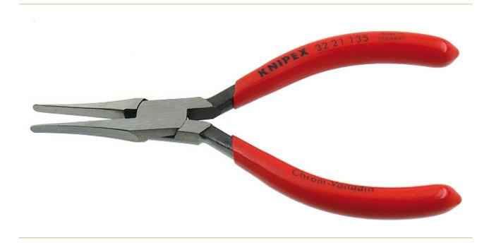
For gripping components and wires with small diameters and for bending contact and relay springs. Polished gripping surfaces. Edges carefully deburred. Flat, wide jaws. - Shape: 2 - jaw thickness (at joint) (D): 7.0mm - tip width (E): 1.0mm - tip thickness (F): 3.5mm - jaw length (B): 34.0mm - head width (A): 12.5mm
