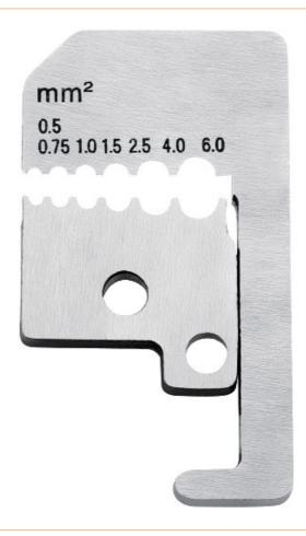
1 pair of spare blades for 12 21 180 With interchangeable blades for four (matched to diameters) or six (matched to cross-sections) different conductor cross-sections. No damage to the conductor due to precisely ground form blades, even fine stranded wires are stripped gently. Clamping jaws hold the wire firmly during stripping. With adjustable length stop for equal stripping lengths when working in series. A pressure spring returns the pliers to their original position.
