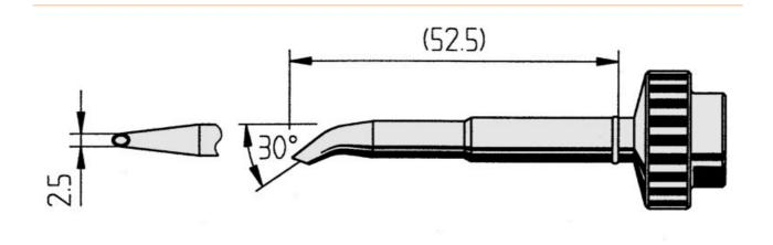
• Permanent soldering tip with ERSADUR-LF coating with increased lifetime for the Tech tool soldering iron, the soldering stations DIGITAL 2000 A, DIGIITAL 60 A and MICRO-CON 60iA
