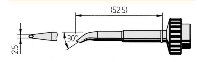
• Permanent soldering tip with ERSADUR-LF coating with increased lifetime for the Tech tool soldering iron, the soldering stations DIGITAL 2000 A, DIGITAL 60 A and MICRO-CON 60iA
