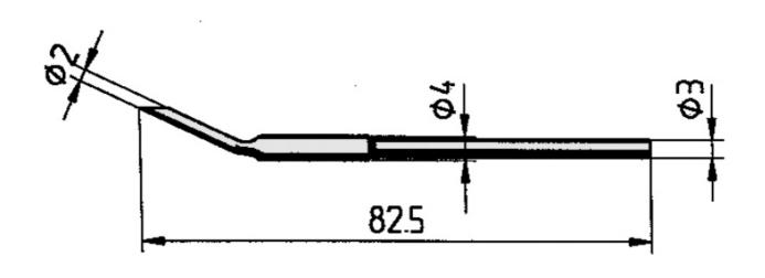
Desoldering tip set for MELF for i-CON, i-CON2 and DIGITAL 2000 A each with desoldering pincette 40 or the CHIP tool, SMT UNIT 60 A/AS, MICRO-CON 60 iA, Rework 80 and SMD 8000 each with desoldering pincette TC40
