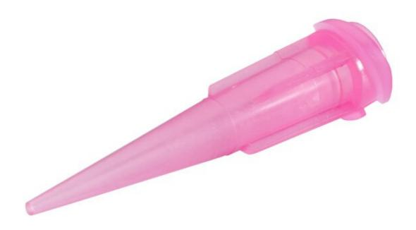
The dosing needle conical, standard, pink, gauge 20, ID= 0.58 mm from Nordson EFD is ideal for use with medium to high viscosity fluids. This Optimum® SmoothFlow™ dispensing needle is made of polyethylene with UV blocker and has a Luer lock thread that ensures a secure and tight connection to the cartridge. With a length of 1.24" and an inner diameter of 0.58 mm, it enables precise and consistent material application. Dispensing tip for cartridge, conical
