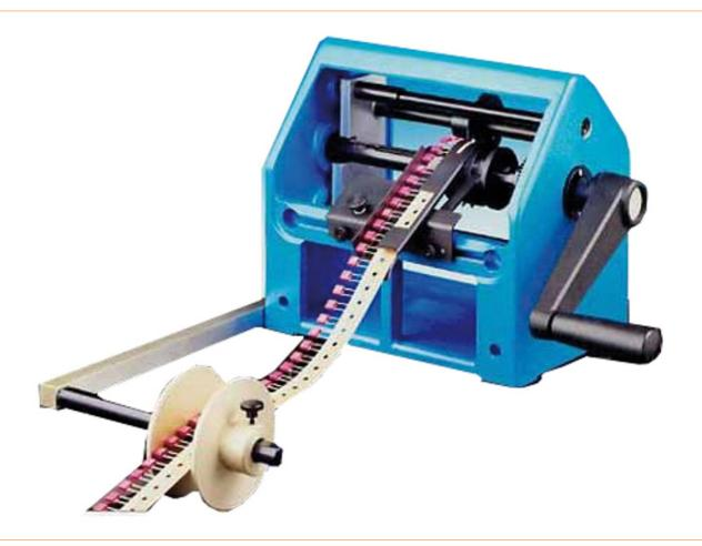
Cutting device for radial components
