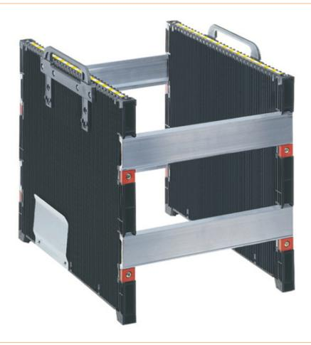
The PCB holders can be loaded in vertical as well as horizontal position. The system is absolutely variable in width and can be mounted for all PCB sizes as required. For the various PCBs, 100, 180 and 300 mm high PCB holders are offered. With 32 guide grooves at 10 mm intervals, the PCB holders offer maximum packing density.
