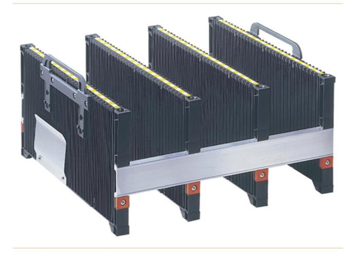
The PCB holders can be loaded both in vertical and horizontal position. The system is absolutely variable in width and can be mounted for all PCB sizes as required. For the various PCBs, 100, 180 and 300 mm high PCB holders are offered. With 32 guide grooves at 10 mm intervals, the PCB holders offer maximum packing density.
