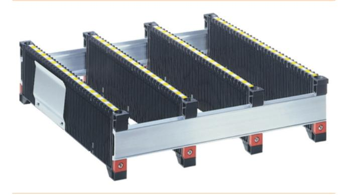
The PCB holders can be mounted in vertical as well as horizontal position. The system is absolutely variable in width and can be mounted for all PCB sizes as required. For the various PCBs, 100, 180 and 300 mm high PCB holders are offered. With 32 guide grooves at 10 mm intervals, the PCB holders offer maximum packing density.
