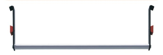
The PCB holders can be assembled in both vertical and horizontal positions. The system is absolutely variable in width and can be mounted for all sizes of PCBs as required. For the various PCBs, 100, 180 and 300 mm high PCB holders are offered. With 32 guide grooves at 10 mm intervals, the PCB holders offer maximum packing density.
