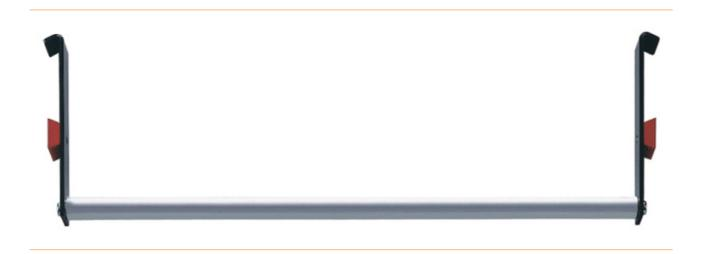
The PCB holders can be mounted in vertical as well as horizontal position. The system is absolutely variable in width and can be mounted for all PCB sizes as required. For the various PCBs, 100, 180 and 300 mm high PCB holders are offered. With 32 guide grooves at 10 mm intervals, the PCB holders offer maximum packing density.
