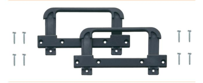
The PCB holders can be assembled in vertical as well as horizontal position. The system is absolutely variable in width and can be mounted for all PCB sizes as required. For the various PCBs, 100, 180 and 300 mm high PCB holders are offered. With 32 guide grooves at 10 mm intervals, the PCB holders offer maximum packing density.
