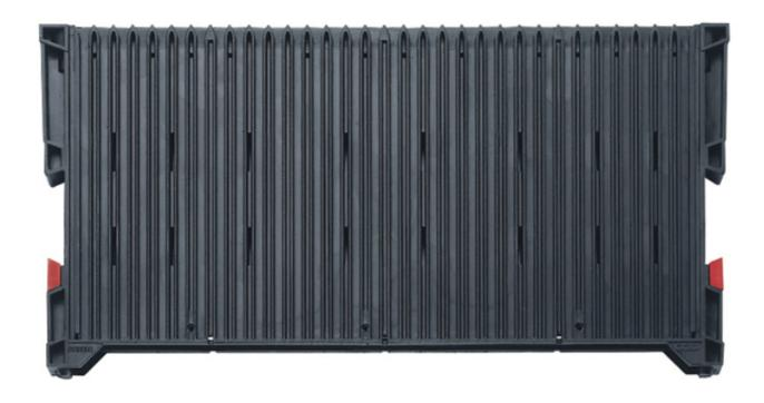
The PCB holders can be assembled in vertical as well as horizontal position. The system is absolutely variable in width and can be mounted for all PCB sizes as required. For the various PCBs, 100, 180 and 300 mm high PCB holders are offered. With 32 guide grooves at 10 mm intervals, the PCB holders offer maximum packing density.
