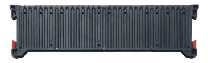
The PCB holders can be assembled in both vertical and horizontal positions. The system is absolutely variable in width and can be mounted for all PCB sizes as required. For the various PCBs, 100, 180 and 300 mm high PCB holders are offered. With 32 guide grooves at 10 mm intervals, the PCB holders offer maximum packing density.
